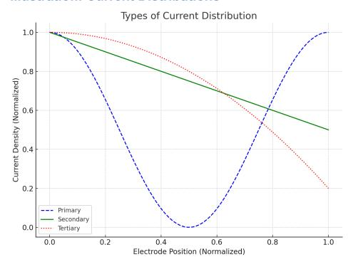
The illustration above compares the primary, secondary, and tertiary current distributions. Primary distribution shows strong geometric influence, secondary considers electrode kinetics, and tertiary includes mass transport effects.
